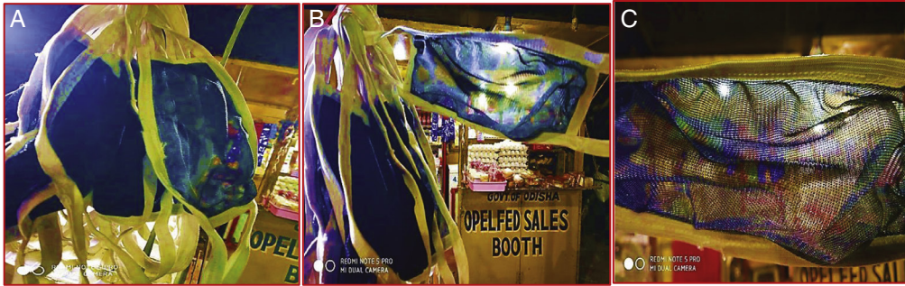
Fig. 3.7 Use of inappropriate mask made up of by mosquito net used in Cuttack, Odisha, India. a) Bunch of homemade inappropriate mask, b) one of the pulled from the bunch and its middle main portion found to be made up of by mosquito net like mesh, c) the pore size of the mask is found to be near about 2 mm. Such masks need to be banned and authorised person must sell mask.
